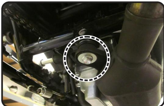
4. Loosen the four header bolts and allow the header to swing forward to where the O2 sensor is accessible.
